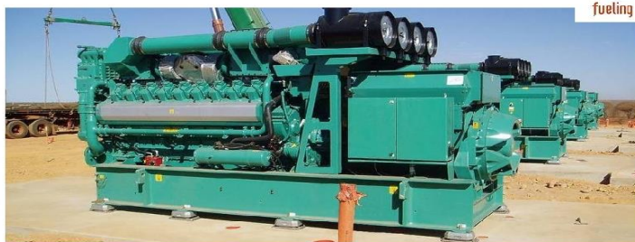
Cummins 750 kW Diesel Generator Set
